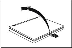
► Press the release button (1) and open the LCD-display panel (2).
