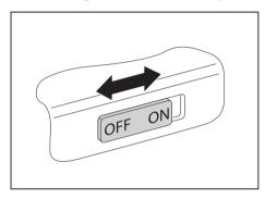
Slide the ON/OFF switch into the "ON" position to activate the radio components.
